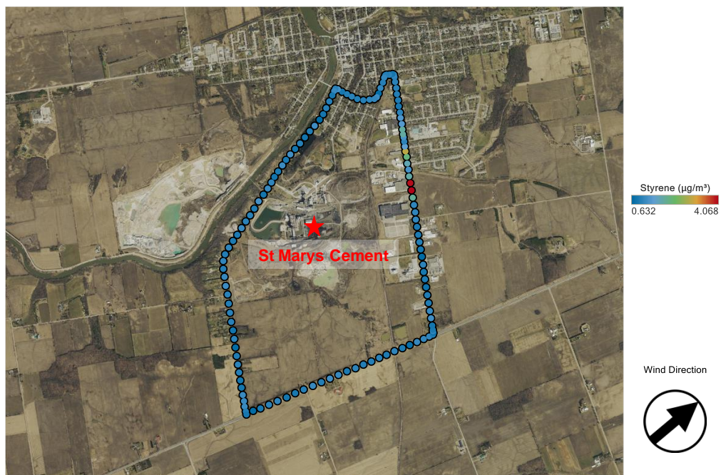
Figure 2: Mobile monitoring of styrene in the vicinity of St. Marys Cement, St. Marys, Ontario, July 17, 2020 09:22-09:34. The arrow indicates the direction the wind was blowing during the measurement period.
