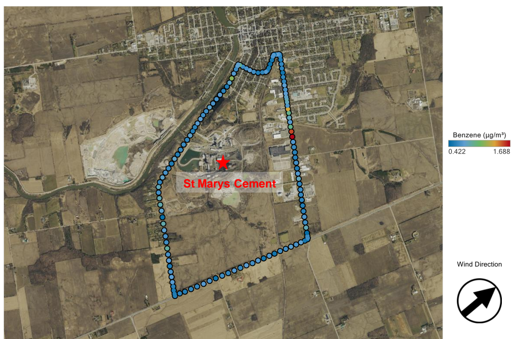
Figure 1: Mobile monitoring of benzene in the vicinity of St. Marys Cement, St. Marys, Ontario, July 17, 2020 09:22-09:34. The arrow indicates the direction the wind was blowing during the measurement period.
