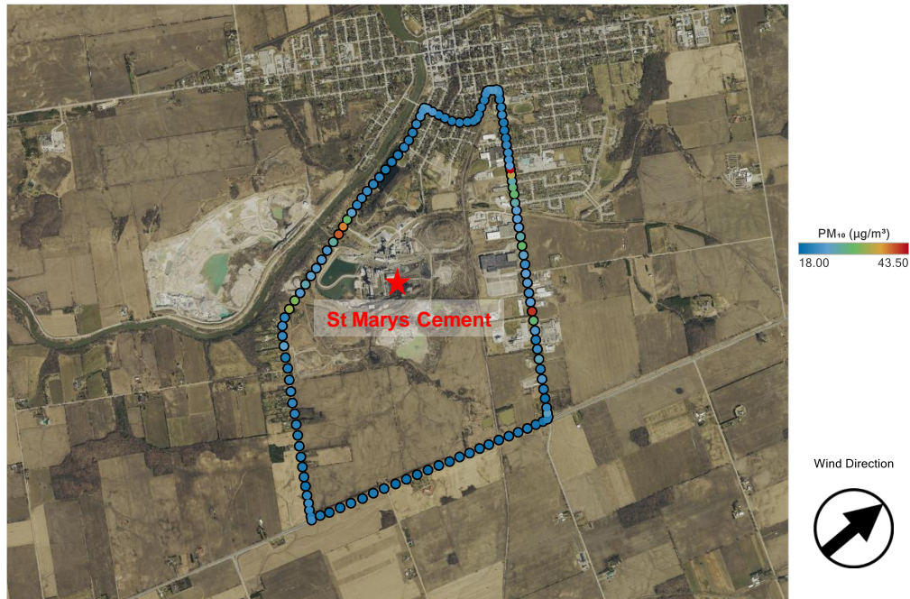
Figure 3: Mobile monitoring of PM 10 in the vicinity of St. Marys Cement, St. Marys, Ontario, July 17, 2020 09:22-09:34. The arrow indicates the direction the wind was blowing during the measurement period.
