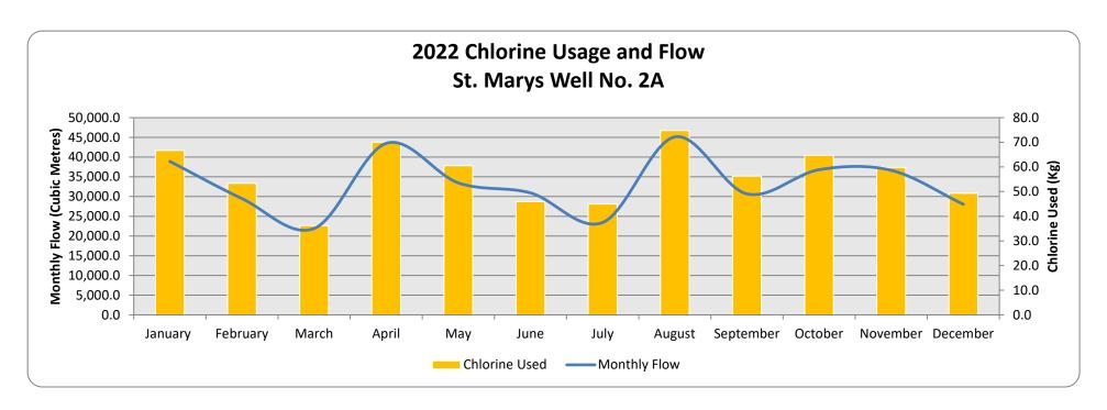
**Monthly Flow** - Total flow volume from the well as recorded by the flow meter **Chlorine Used** - Total amount (Kg) of Chlorine used during each month at the well
