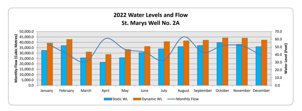
Monthly Flow - Total flow volume from the well as recorded by the flow meter
