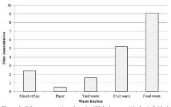
Figure 2. Olfactometery values from landfill lysimeters with the individual MSW fractions.
