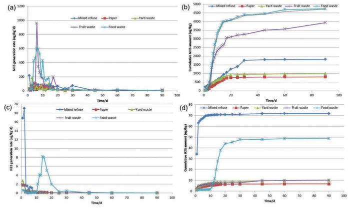
Figure 1. The generation rates and the cumulative amounts of NH<sub>3</sub> and H<sub>2</sub>S from landfill lysimeters.
